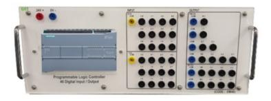
EPT200 is a advance PLC learning kit suitable for variety brand with built-in power supply, 4mm socket/phoenix contact, simulation indicator lamp, toggle switch, analog IO, HMI, operation start/stop/Estop button etc
